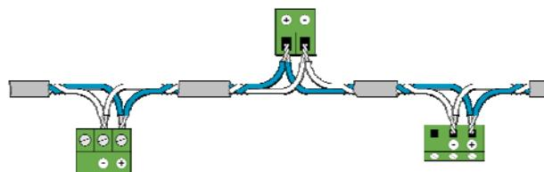
The potential difference of all bus members must not exceed  $\pm 7V$ . Therefore the use of a shield or of a third wire (ref line) for potential equalization is recommended.
