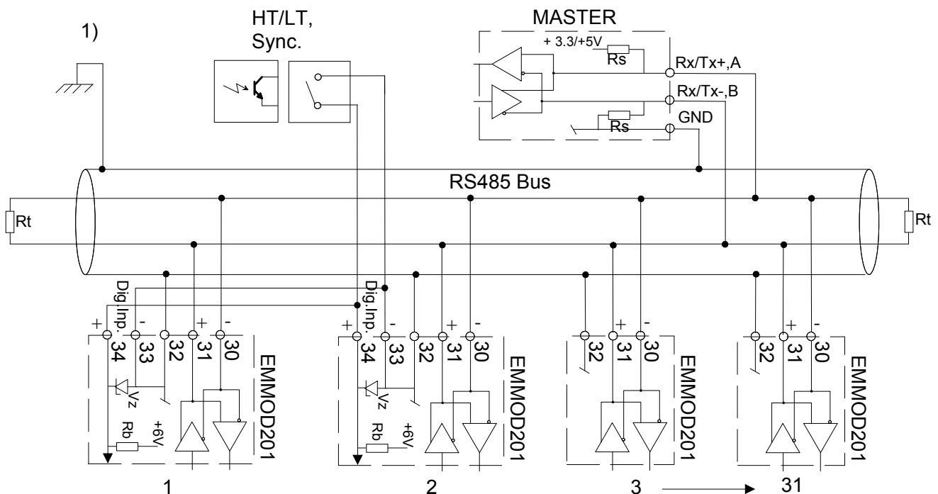
All devices must use the same bus settings (baudrate, parity control) but a unique device address. These settings may be performed locally at the device or via RS232 interface.
