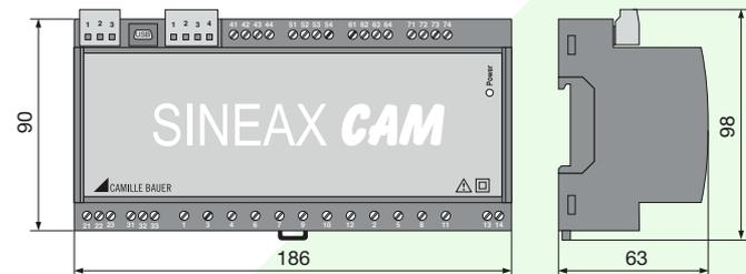
SINEAX CAM in housing clipped onto a top-hat rail (35 x 15 mm or 35 x 7.5 mm). Terminals partly pluggable.
