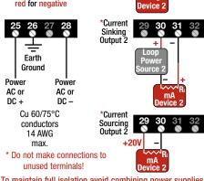
To maintain full isolation avoid combining power supplies in common with inputs, outputs, or unit power.
