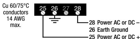
To maintain full isolation avoid combining power supplies in common with inputs, outputs, or unit power.
